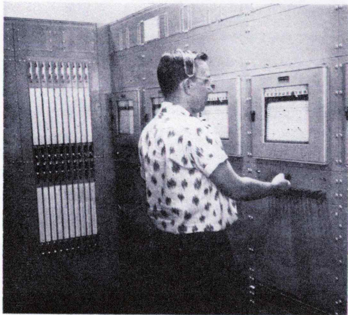
Fig. 6—The operator is here shown recording the output of a single measuring gage under calibration. Since the recorders in measuring calibration are used as a load on the measuring gages, substituting for the telemeter subcarrier oscillators, the value of the input impedance of the recorders has been changed to correspond to this. To the left is seen a "harp" bank. In each panel in the bank is a set of individually isolated horizontal and vertical wires which may be interconnected by means of a small clip. By using this bank, any wire on any incoming cable from the missile may be connected to any individual recorder point in the whole room. The bank shown has the possibility of 162,000 different connections, thus providing maximum flexibility in minimum space. Facilities for patching into the building communication system are provided below the recorders.
