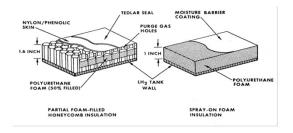
with helium gas, intended to preclude atmospheric moisture from condensing and freezing on the outside metal tank surfaces. The second, and much improved design, used sprayed-on foam that adhered better and provided significantly improved resistance to heat transfer. It was used on most flights after Apollo 11.
