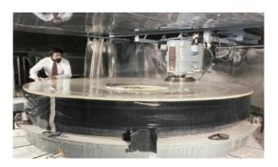
compressed. The photo shows the primary mirror being polished at the P-E plant in Danbury, Connecticut.
